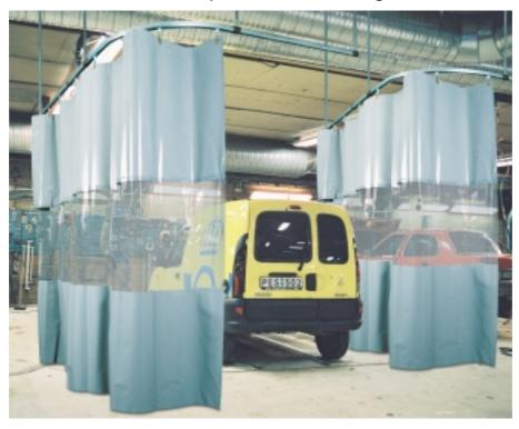
Workplace screening used for welding/grinding jobs at car repair or car body shops. Customized curtain size. The opaque fabric is flame and tear resistant PVC-coated polyester; the fully transparent fabric is flame-resistant, softened PVC. For exact colour rendering, ask for our colour samples.
