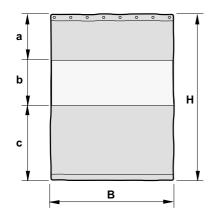
Standard curtain fabric is supplied with eyelets c/c 400 mm at the top.
