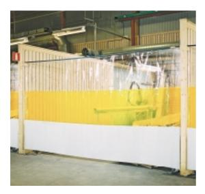
Welding curtains mainly used for screening off welding/grinding workplaces. Curtains are customized. The opaque fabric is flame and tear resistant PVC-coated polyester; the fully transparent fabric is UV-absorbing and flame-resistant.
