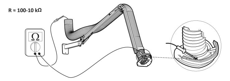
If tested as above with accurate multi meter, normal resistance should be between 100-10 k $\Omega$ . Maximum resistance shall not exceed 100 K $\Omega$ .
