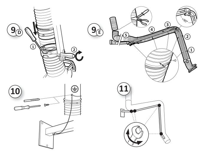
10) Secure the hose to the existing air duct with the accompanying clamp and screw the hose's ground connection to the air duct. Ensure that proper electrical contact is made.
