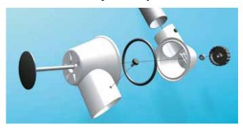
Terfu joint. The large frictional diameter together with the single grip adjusting knob provide a rigid, stable joint with a smooth easily adjustable function without requiring the application of excessive force or tools. The joint has reinforced side pieces. Ball bearings that isolate the adjusted friction level allow the arm to move up and down without locking the joint or loosing stability and function.
